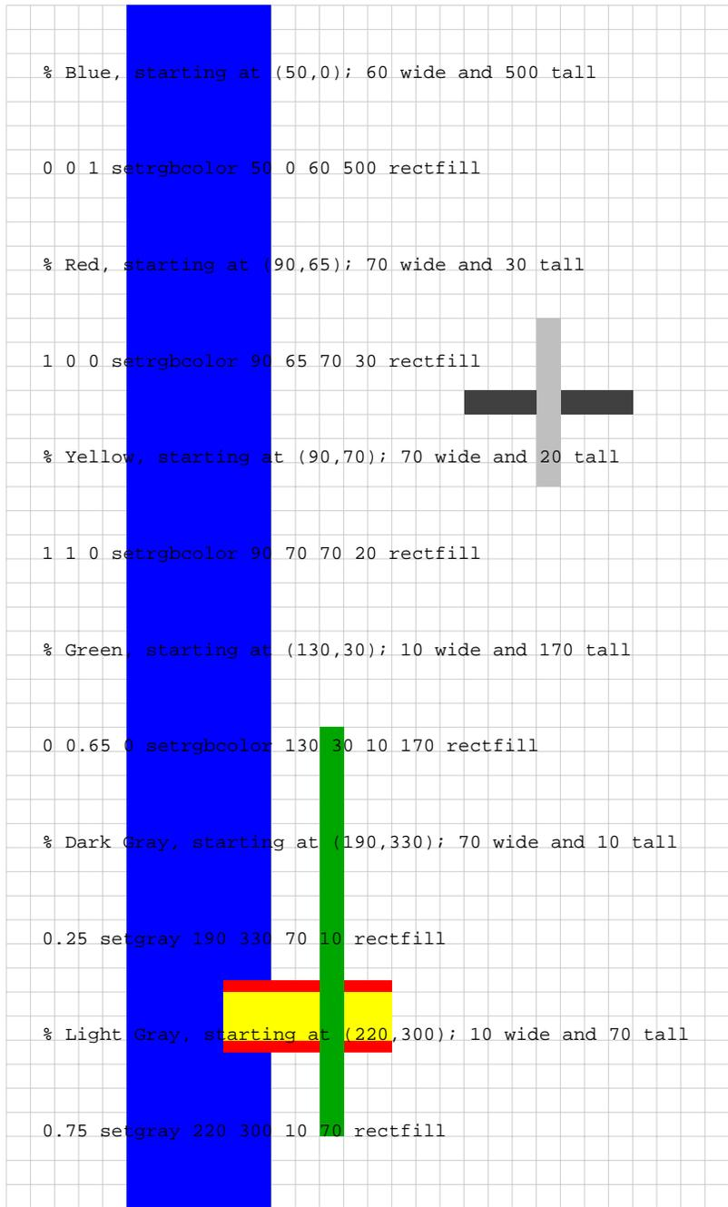
The image shows a grid with several colored rectangles drawn on it. A large blue vertical bar is on the left. To its right, there is a red horizontal bar, a yellow horizontal bar, a green vertical bar, a dark gray horizontal bar, and a light gray vertical bar. The code on the left side of the grid describes the position and size of each rectangle.
