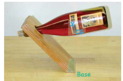
This wine bottle holder is stable because the CG is right over the base of support.
