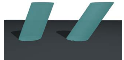
The base of support for these tilted cylinders is the area where they are in contact with the floor.
