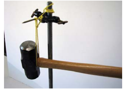
The center of gravity of the hammer is located inside the handle close to the hammer's head.
