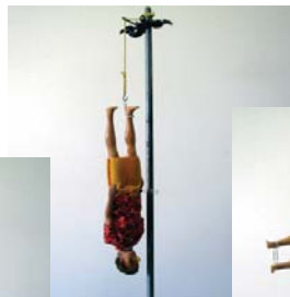
The doll has a hollow head so its CG is located a bit lower in the body than for a human.
